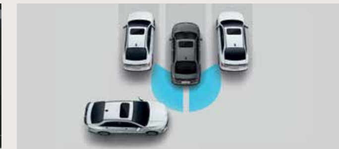
Rear Cross - Traffic Collision - Avoidance Assist (RCCA) & Rear Cross - Traffic Collision Warning (RCCW)
