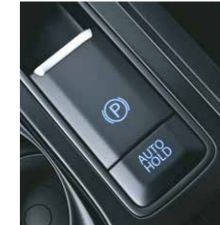
Electric parking brake (Turbo only)
